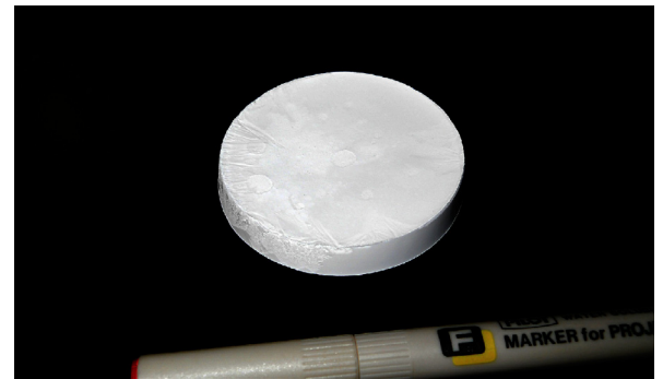
Top: Ice binding model of the fish type II AFP (JMB 383(3), 734 (2008). Middle: AFP powders produced by a licensed company (Red tags) and this lab (Right). Bottom: “A high porosity ceramics” prepared by utilizing the supreme ice shaping ability of AFP.
